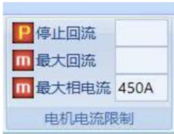
For the electronic brake function, when braking, the vehicle will give a braking signal to the controller. After the controller detects the braking signal, it will perform electronic braking with the current that stops the return flow, and the braking current does not exceed the maximum return value.
